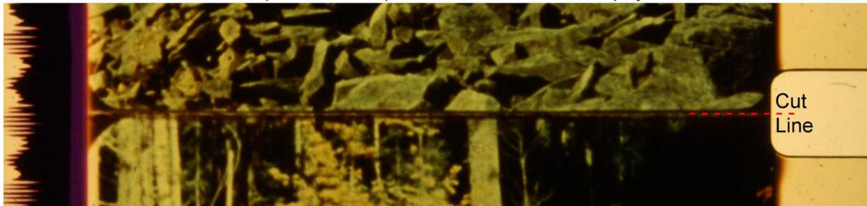
**Figure 2B.** Technique sometimes referred to as an "Invisible Splice". While the "invisible splice" technique does remedy the tape line in the film image area, it does not remedy the cut line and the prospect the cut line will allow a light leak onto a copy which is printed by continuous contact printing machinery. As such, the splice may not actually be invisible on examination of a copy.
