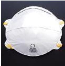
Disposable particulate respirators are sometimes confused with “dust masks” but are distinctly different. A disposable respirator has been tested by the National Institute of Occupational Safety and Health (NIOSH) to make sure it can remove very small particles. A disposable respirator only removes particles. It does not remove gases, chemicals, or vapors from the air you breathe.
