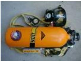
This type of respirator supplies clean air directly to the user from a cylinder worn on the back of the user containing Grade D breathing air. Most cylinders are rated to last 30 to 45 minutes depending on size and breathing rate.
