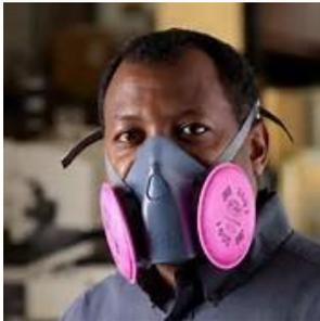
Respirator with particulate filters capture particle in the air, such as dusts, mists, and fumes but do not protect against gases or vapors. Filters should be replaced when user finds it difficult to breathe through them.
