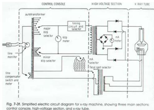
Fig. 7-31. Simplified electric circuit diagram for x-ray machine, showing three main sections: control console, high-voltage section, and x-ray tube.
