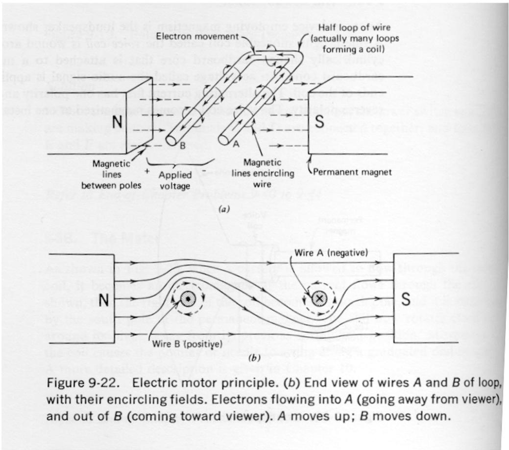
Figure 9-22. Electric motor principle. (b) End view of wires A and B of loop, with their encircling fields. Electrons flowing into A (going away from viewer), and out of B (coming toward viewer). A moves up; B moves down.
